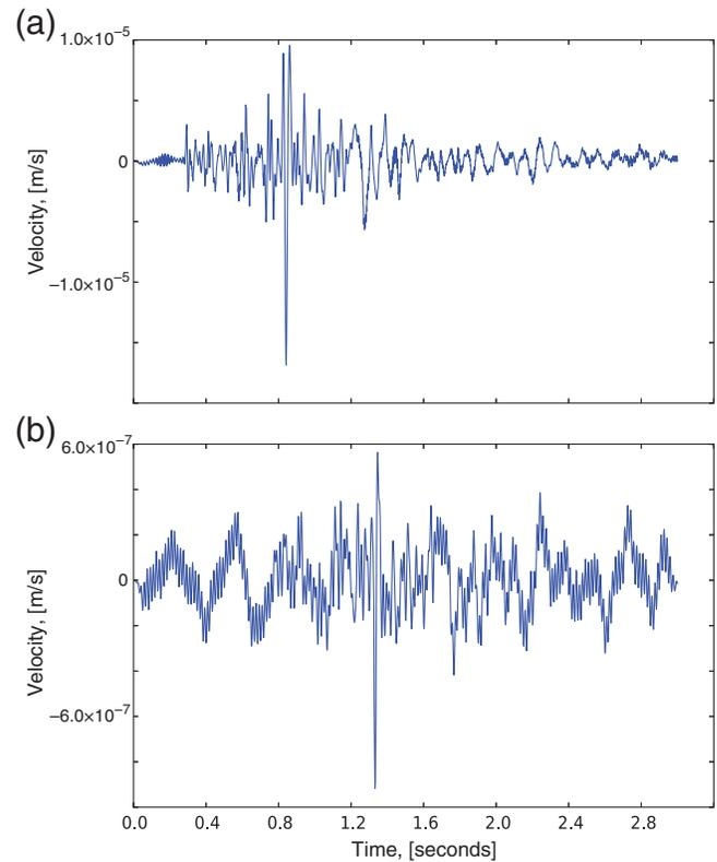
▲ **Figure 2.** (a) Velocity trace from the vertical shallow borehole channel at station DEC03 for an event with  $M_w$  0.86, with instrument response removed. (b) Velocity trace from the vertical shallow borehole channel at DEC03 for an event with  $M_w$  0.23, with instrument response removed and band-pass filtered from  $1.0$  to  $55$  Hz.
