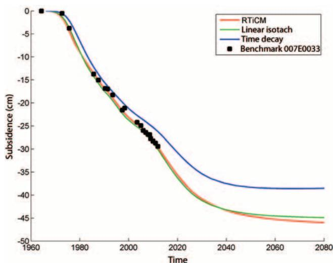
**Figure 3.** Different compaction models (RTiCM, linear isotach, and time decay) and their fit to a leveling benchmark in the center of the field.
