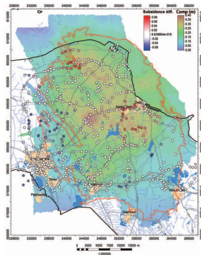
**Figure 4.** Compaction in the Groningen reservoir in January 2012, calculated with the RTCM model. The difference between calculated and measured subsidence is indicated in colors at the benchmark locations (labeled "Subsidence diff."). Red indicates that the calculated subsidence is larger than the measured subsidence. After TNO (2013b), Figure 5.13. Used by permission of TNO.
